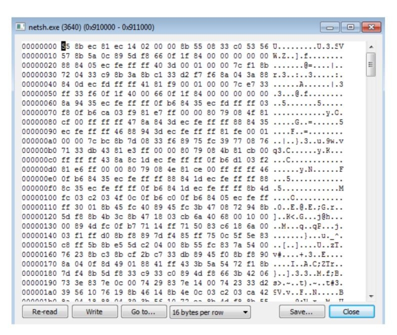
Finally, the "TokyoX" loader runs from the DLL (version.dll) in netsh.exe through the API NtcreateThreadEx and we see the start of the last page created in the stack:
