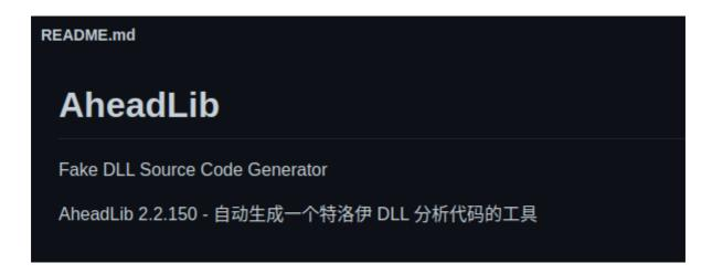
Basically, this tool will allow you to create a C++ source code file, implementing a DLL with the same exported functions as a given DLL. For the purpose of the current analysis we generated a source code file using this tool and giving the legitimate version.dll as input.
