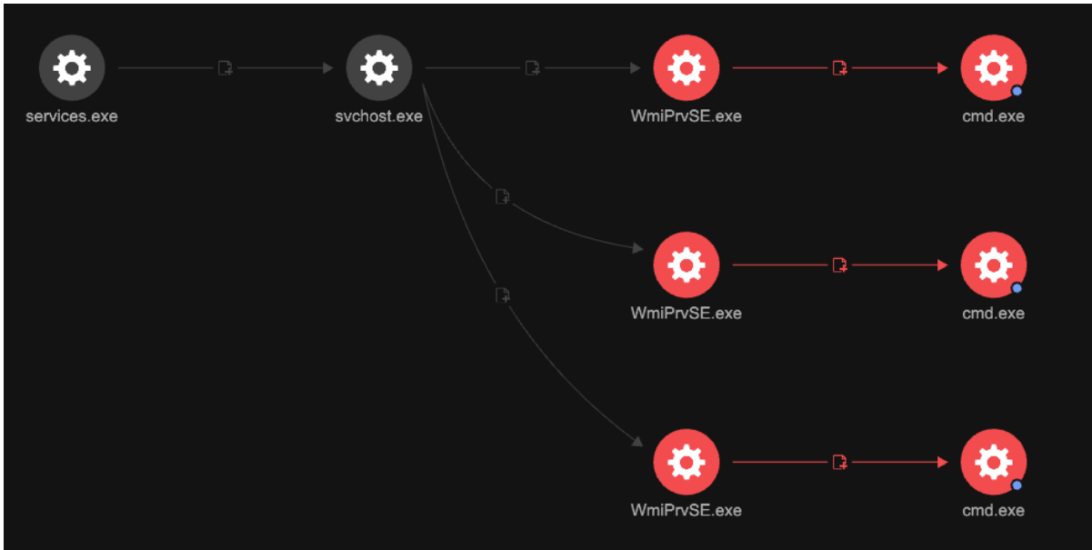
Figure 8. Execution profile for Buer Loader's malicious document on the Trend Micro Vision One console
