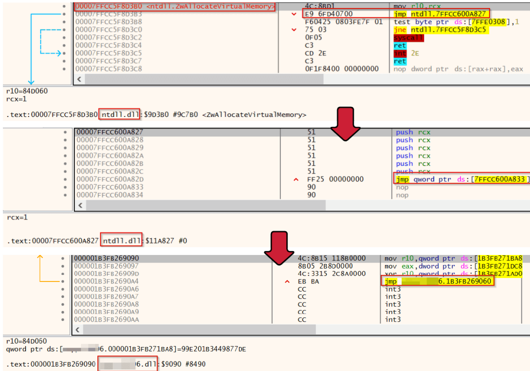
The figure shows that the Native API NtAllocateVirtualMemory (Zw) is hooked inline ( jmp ) by the EDR and redirects to the hooking.dll from the EDR
