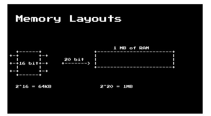
The 8086 CPU is a 16 bit CPU, but with 20 bits of memory addressing. This means the CPU can only hold values that point to 64KB, this is a problem when the memory space is up to 1MB.
