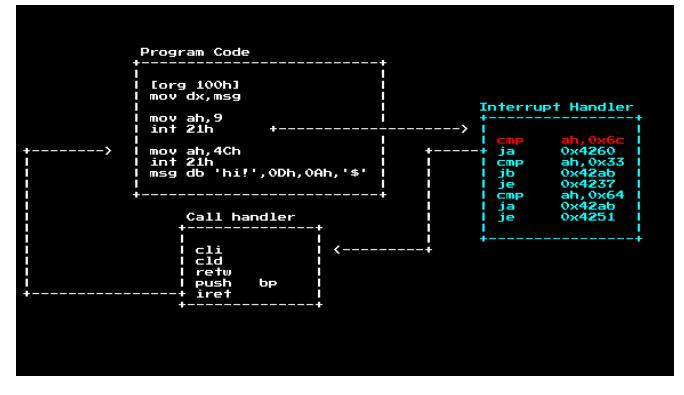
We do this because the Interrupt handler is always in a fixed location in MS-DOS (this is way before the era of <u>ASLR</u> and Kernel ASLR) and the program location is not.
