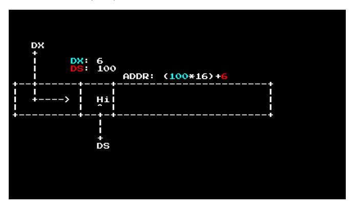
In the case of this call DS is used as a pointer inside the 16 bit window as to where the start of the string is. The string printer will then scan until it finds a \$ symbol and then stops. This is similar to other systems that use a null byte instead of a \$.
