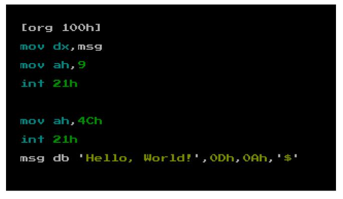
As we can see there are two int calls here. We use 21h (h = hex) as the master syscall number, and we can specific what action we want MS-DOS to do based on the value of Ah
