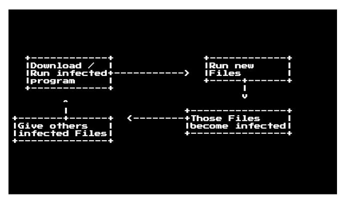
Once you have got an infected file on your system and run it, the malware will either actively search or install syscall hooks to programs you run after. It will often do this in a subtle and non visible way to avoid detection. The importance of subtlety is important since to spread
