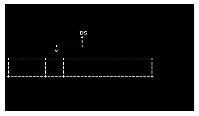
This is allows a 16 bit CPU to see all 20 bits of RAM, by ensuring that for every value of DS, the window is shifted by 16 bytes.
