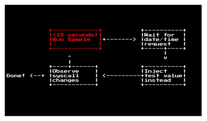
The sample testing stage takes around 15 seconds since it is using a full qemu emulation process, and it could take up to 15 seconds for the program to fully run in the VM. Since DOS does not have power saving features, this means when DOS is idle, it is in a <u>busy loop</u>
