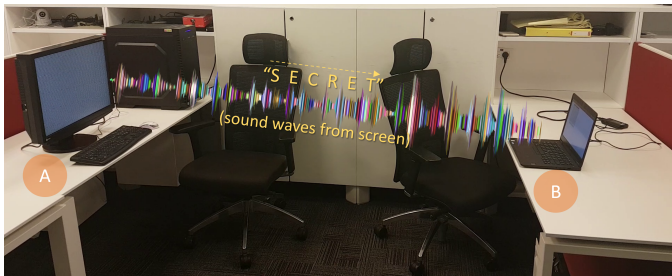
Fig. 1. Attack scenario. A malware infection on the compromised computer (A) encodes information and uses crafted pixel patterns to exfiltrate it over the emanated acoustic signals. A nearby laptop computer receives the signals, decodes them, and sends them to the attacker.
