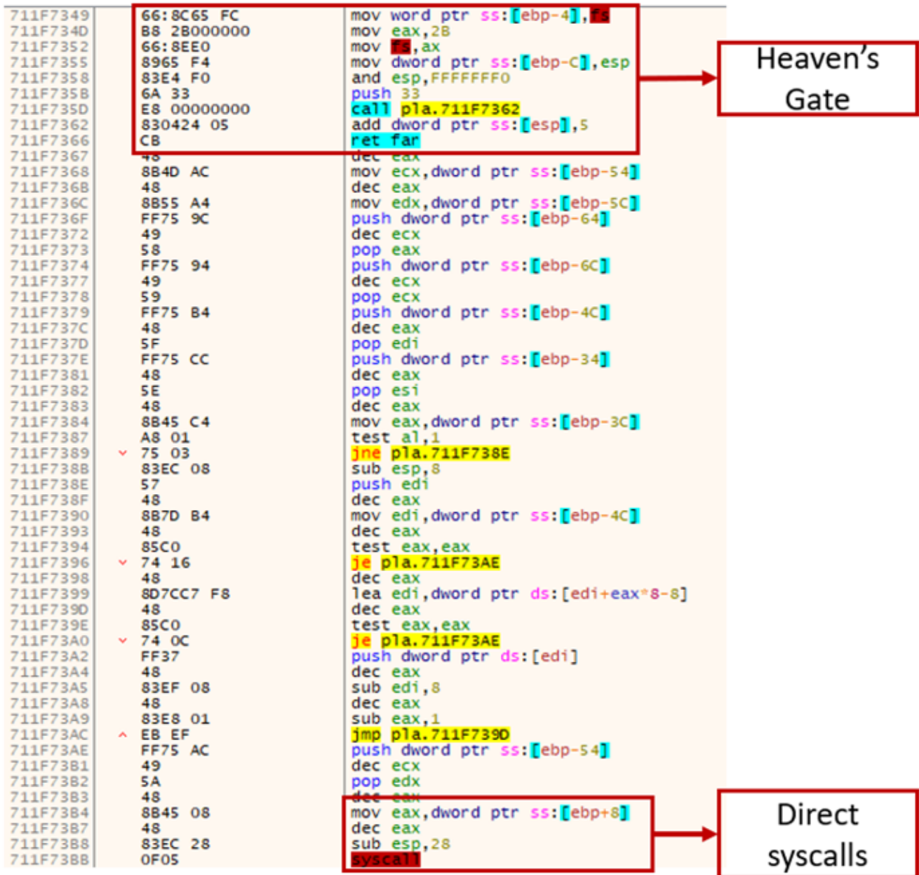
Figure 8: Using heaven's gate and direct syscall for the injection.
