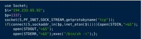
Figure 2: The initial payload that creates a reverse shell to Kinsing's C2 server
