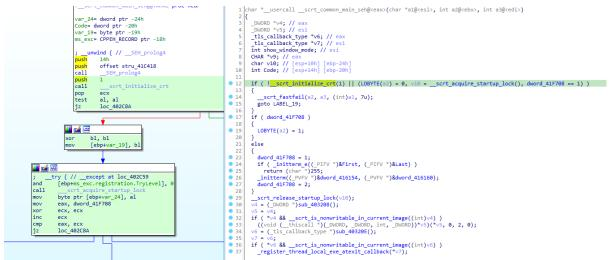
It checks for CPUID and if processor feature *PF\_XMMI64\_INSTRUCTIONS\_AVAILABLE* is present on the impacted system. If enabled, the malware knows that the SSE2 instruction set is available and more complex mathematical operations are possible.
