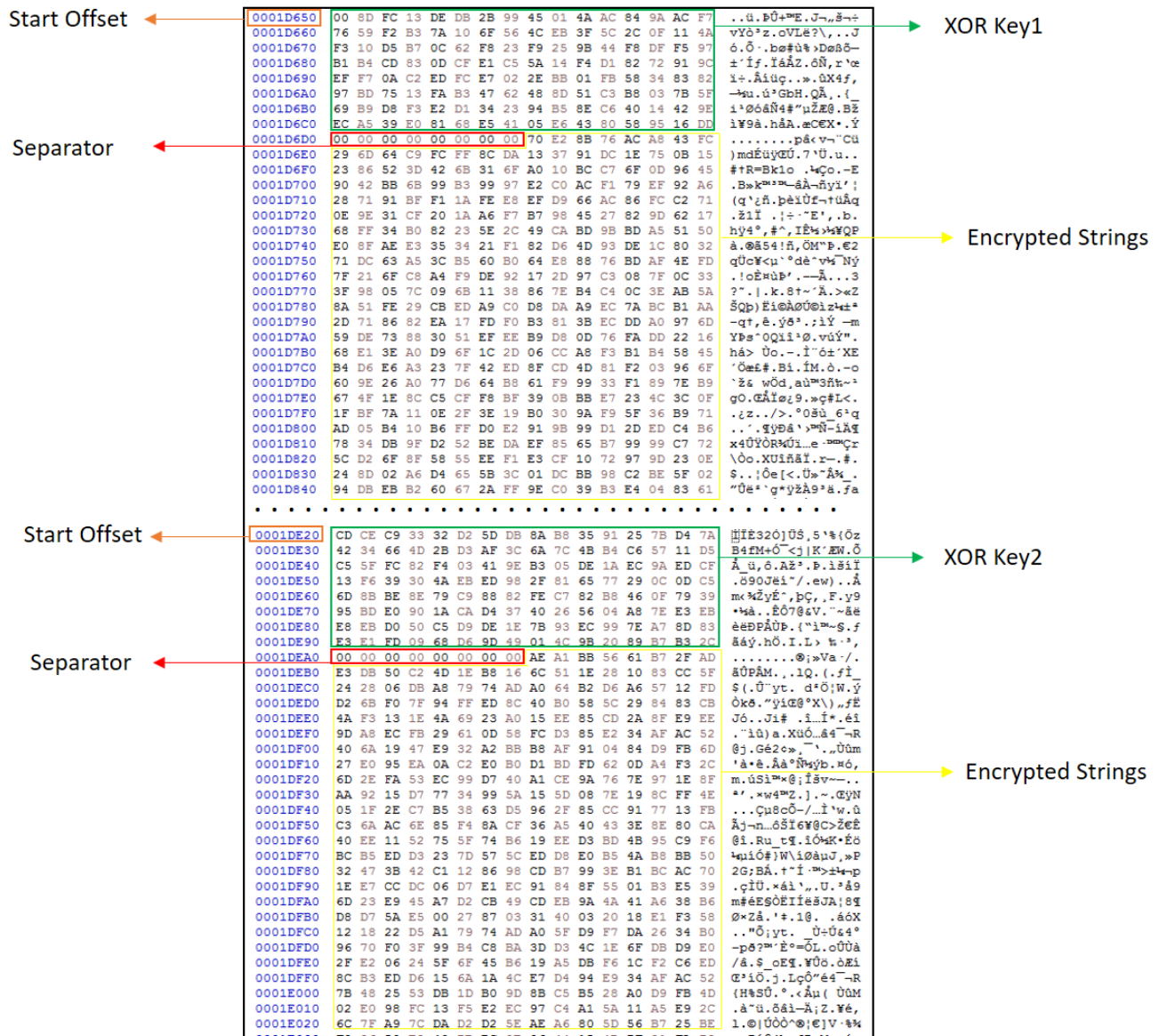
Figure 13 -Shows the encoded strings residing in the .DATA section of the Qakbot malware.
