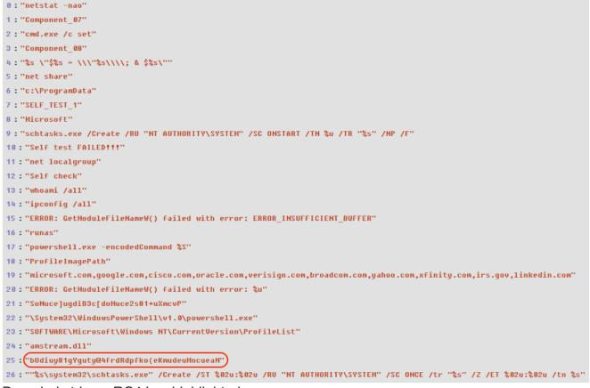
Decoded strings: RC4 key highlighted
