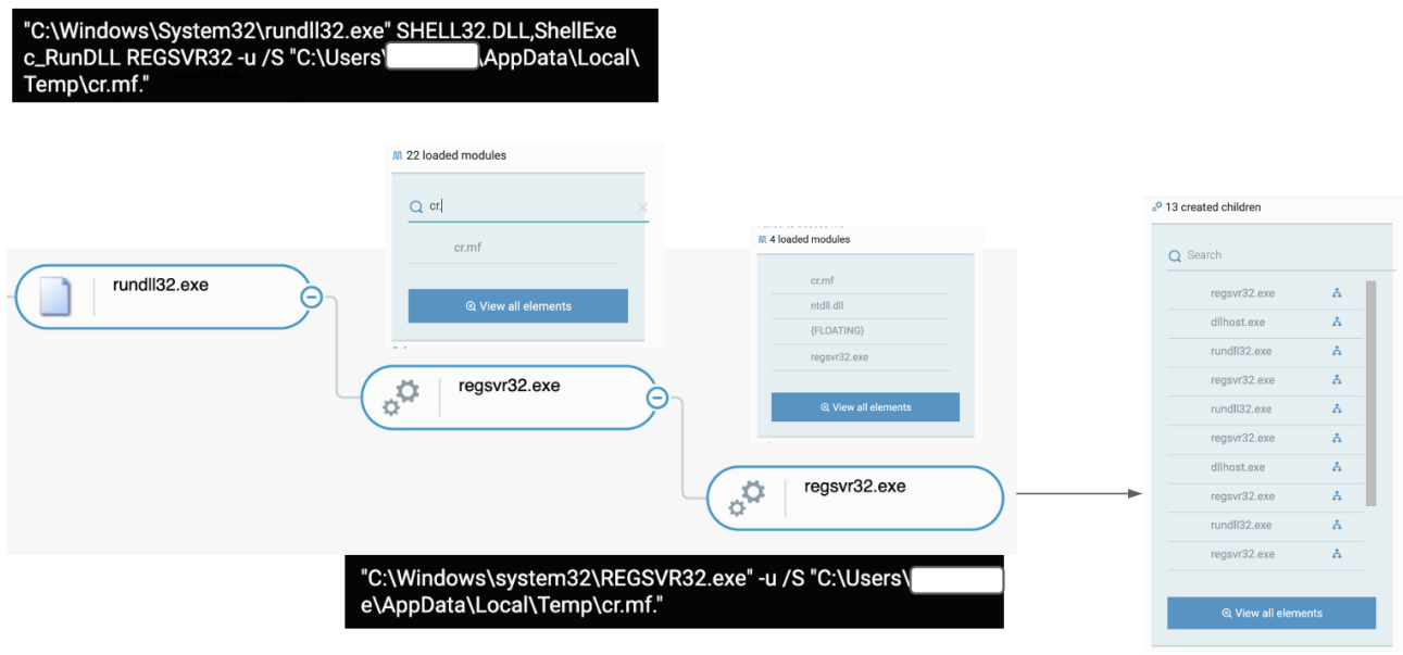
Process tree showing the persistence mechanisms used by Raspberry Robin as seen in the Cyberreason Defense Platform
