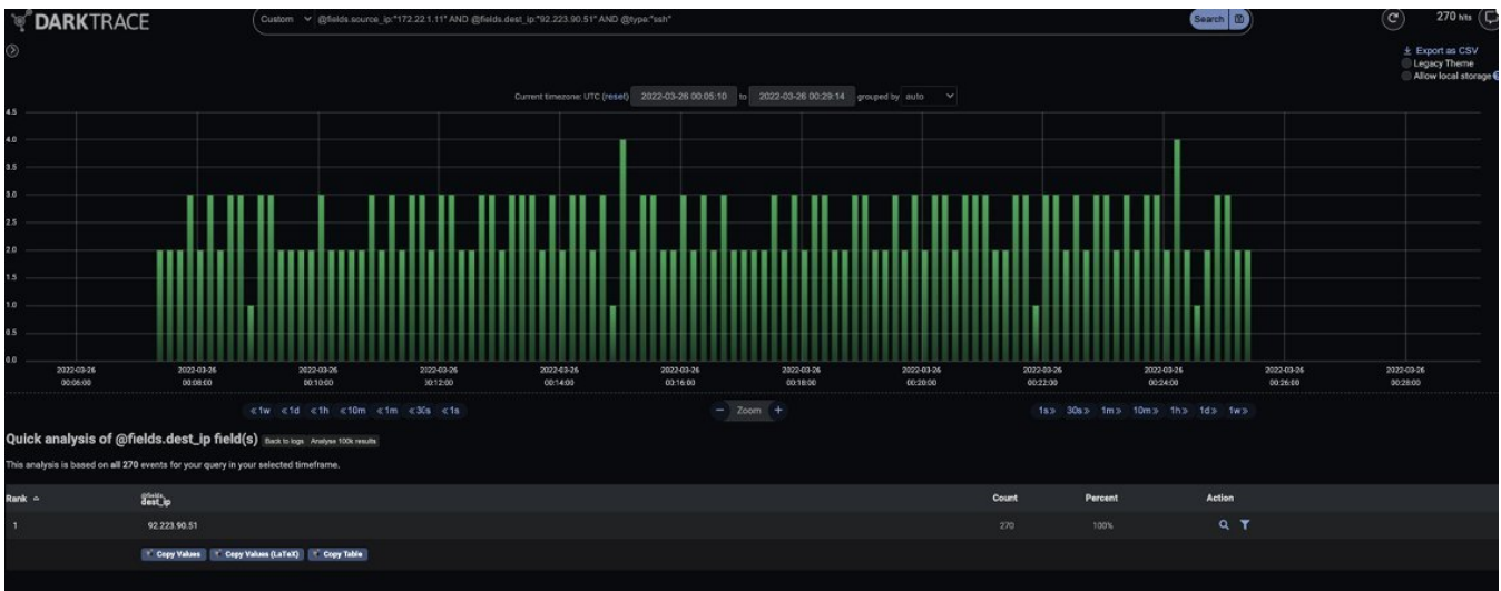
Figure 10: Beaming SSH connections to a single external endpoint, indicating a potential brute-force attack
