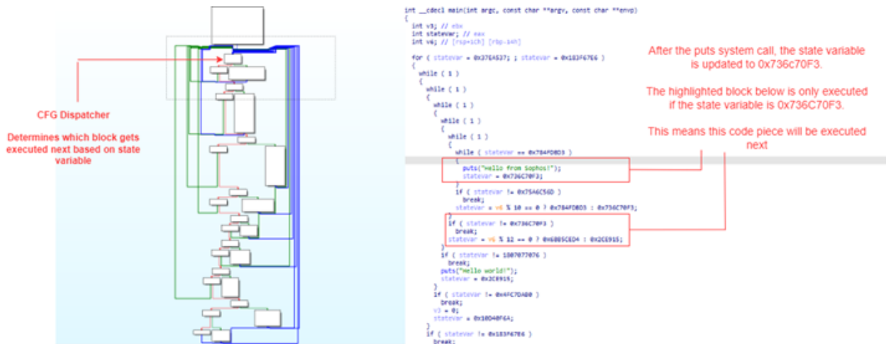
Figure 4: Annotated example of a flattened function
