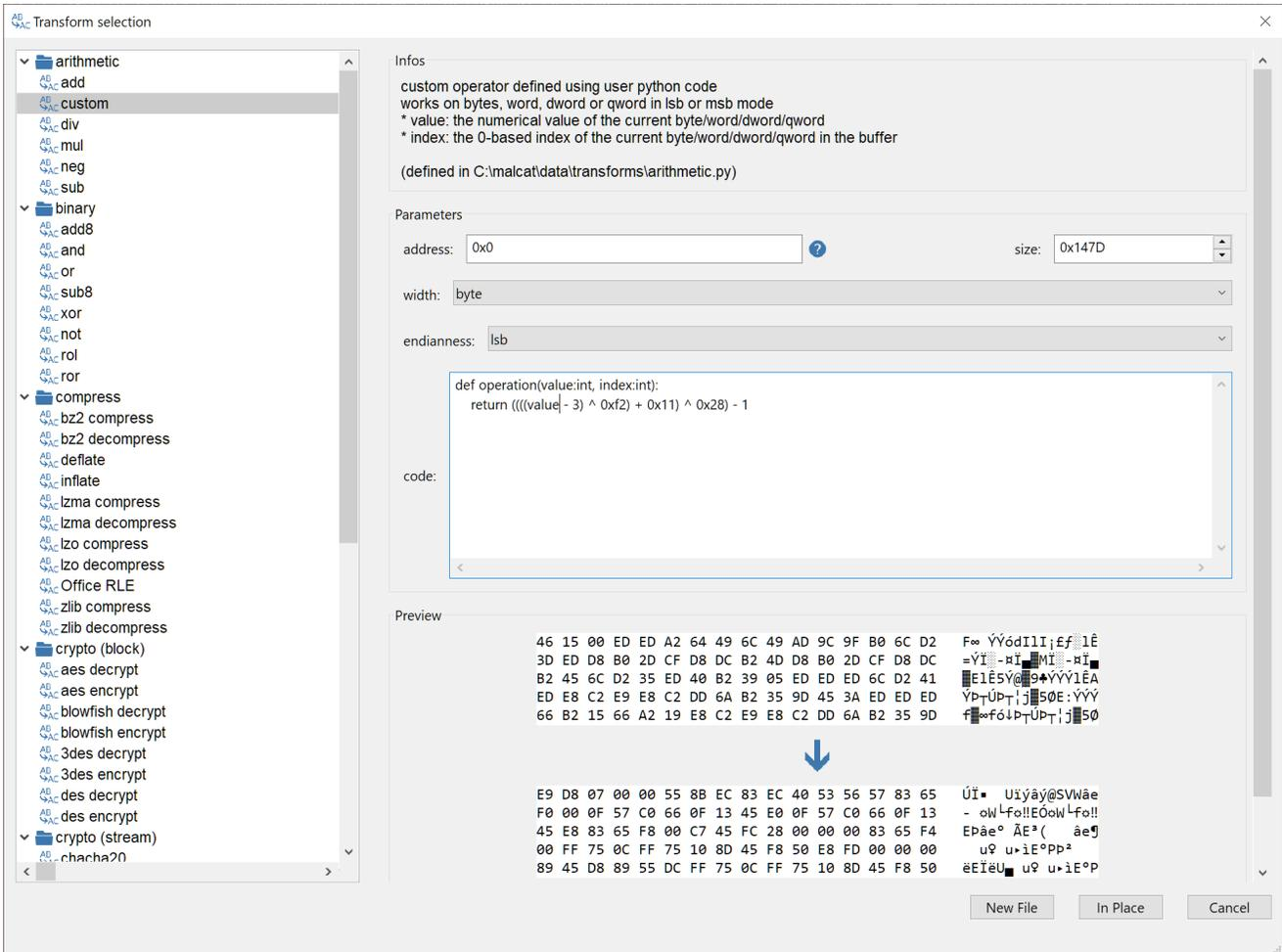
Figure 6: decrypting the shellcode
