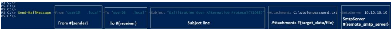
Figure 8 — Victim host sends stolen data to the attacker-controlled email box using SMTP. Figure 9 shows the ‘Successful Email Delivered’ to the attacker’s email box:
