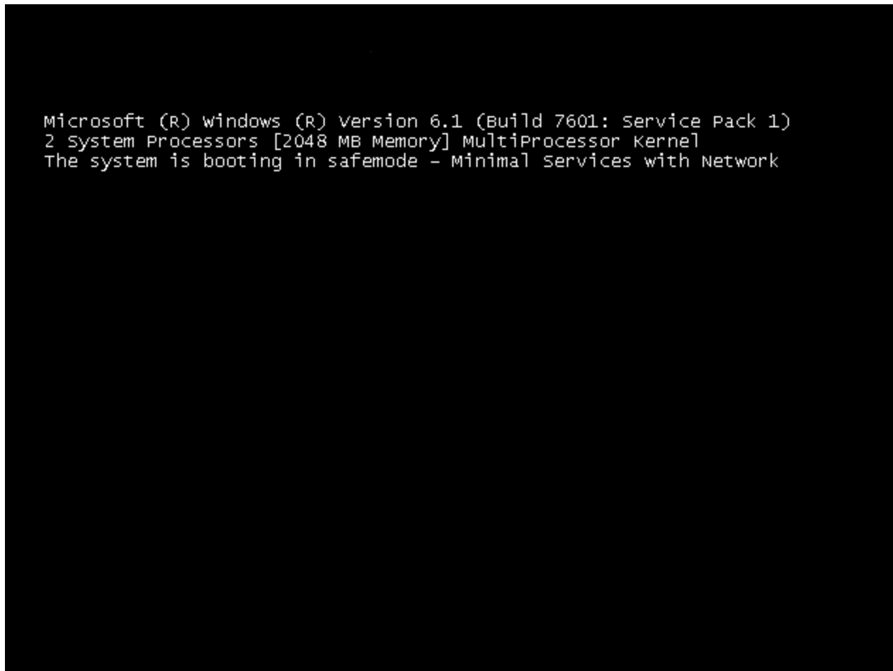
Figure 2. Conti booting Windows into Safe Mode with networking enabled to encrypt files
