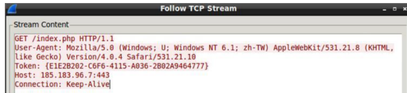
Figure 5 - Screenshot of the GET request sent over port 443 for "index.php" from the IP address 185[.]183[.]96[.]7.
