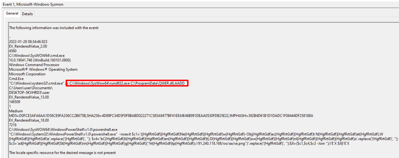
Figure 15: Powershell execution to run malicious DLL files with arbitrary arguments As shown in the red box in figure below, at the end of the script, the script will execute the command to begin the DLL binary execution.
