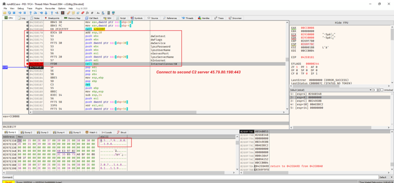
Figure 27 : Malware making second connection to another C2 server, 45.79.80.198 Initiating the request of the connection will create the connection as Netbytesec malware analyst observe the network behaviour and step over the HttpSendRequest function.
