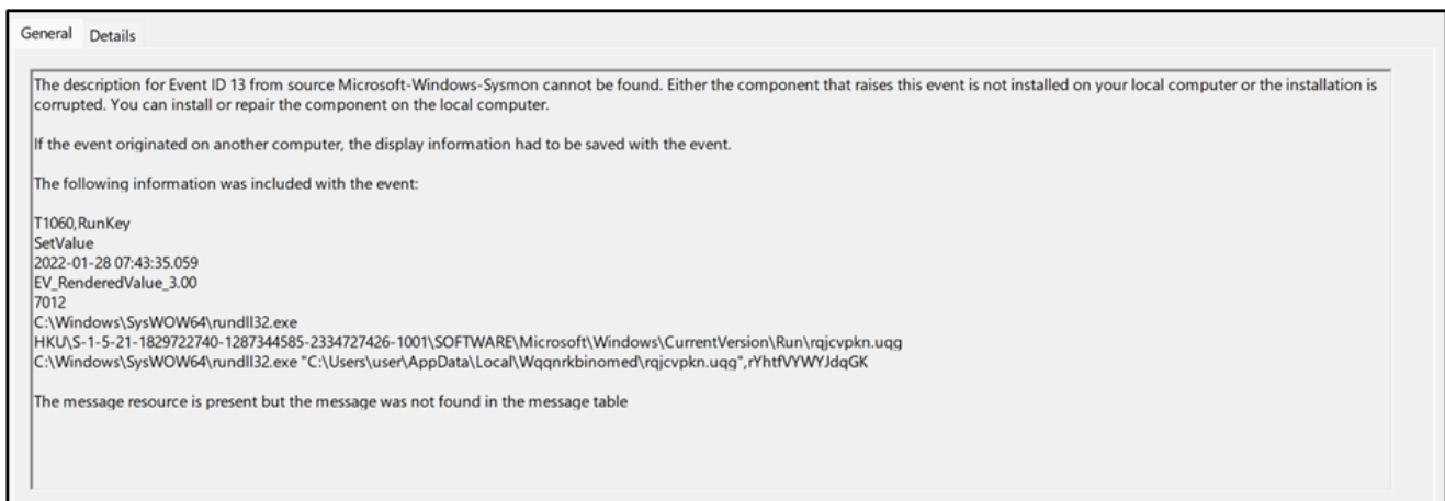
Figure 21: Malware attempt to register at startup of the windows as persistence mechanism, with alongside new binary with new arguments at new path
