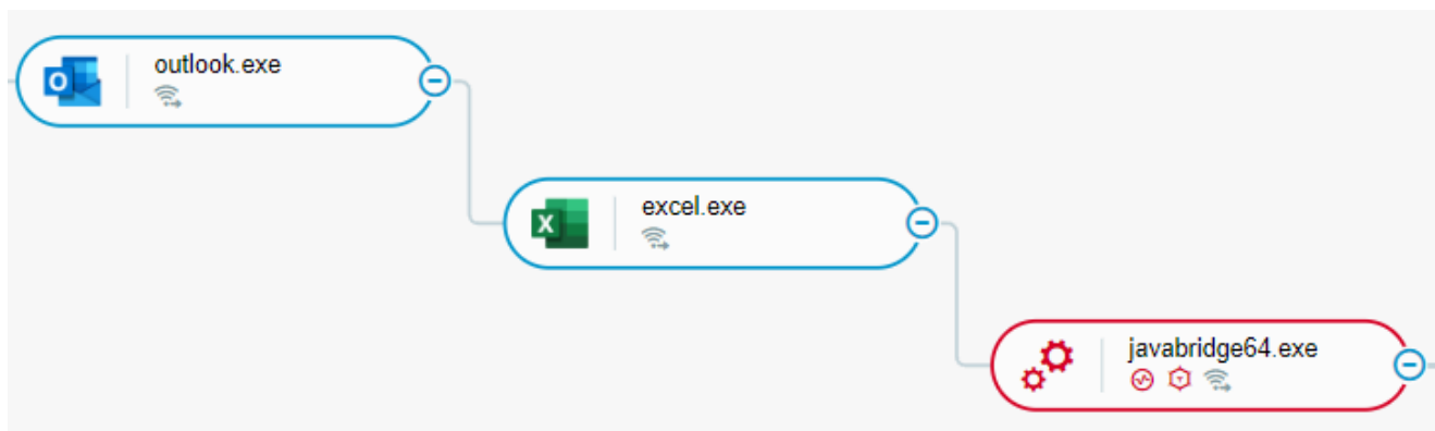
Malicious Office macro executes IcedID javabridge64.exe as seen in the Cybereason XDR Platform
