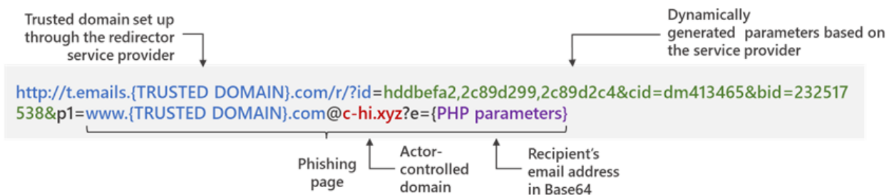
Figure 4. The actor-controlled domain uses a DGA pattern and a .XYZ top-level domain
