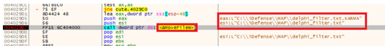
Figure 16 Malware Replaces Original Content with Encrypted Content
