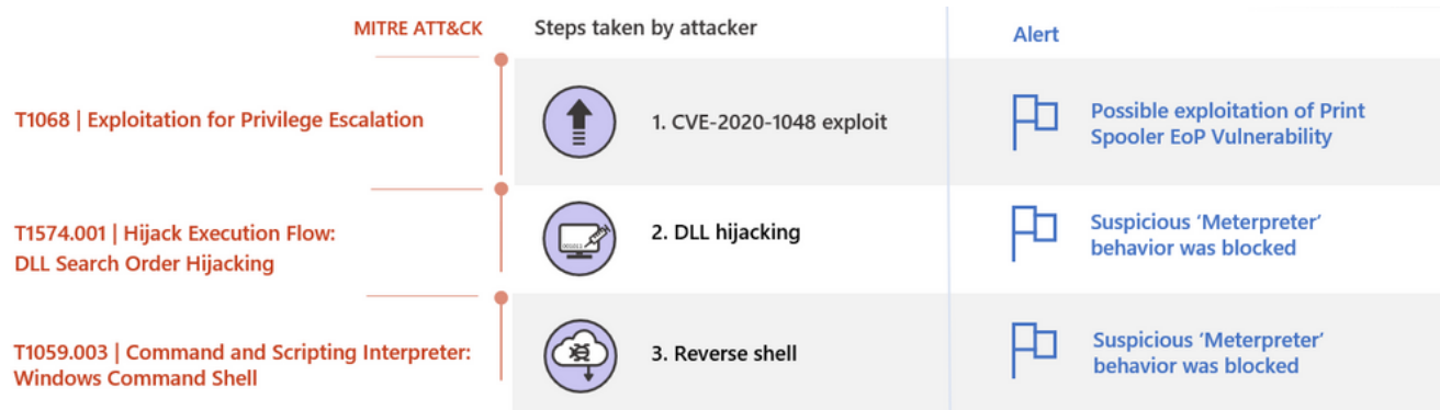
Figure 20. MITRE ATT&CK techniques and alerts flagged for each attacker step
