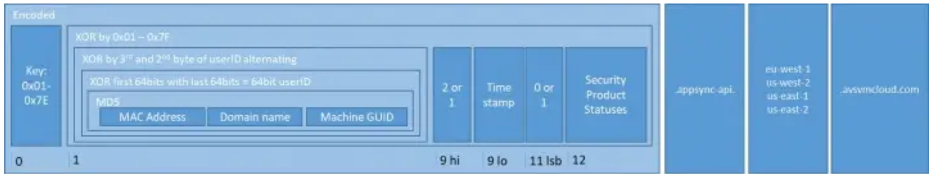
Figure 2. Structure of second DNS lookup communicating security product status The responses to these DNS queries may then contain control information for the threat to terminate or launch a secondary HTTP communication channel, something that we plan to cover in a subsequent blog.
