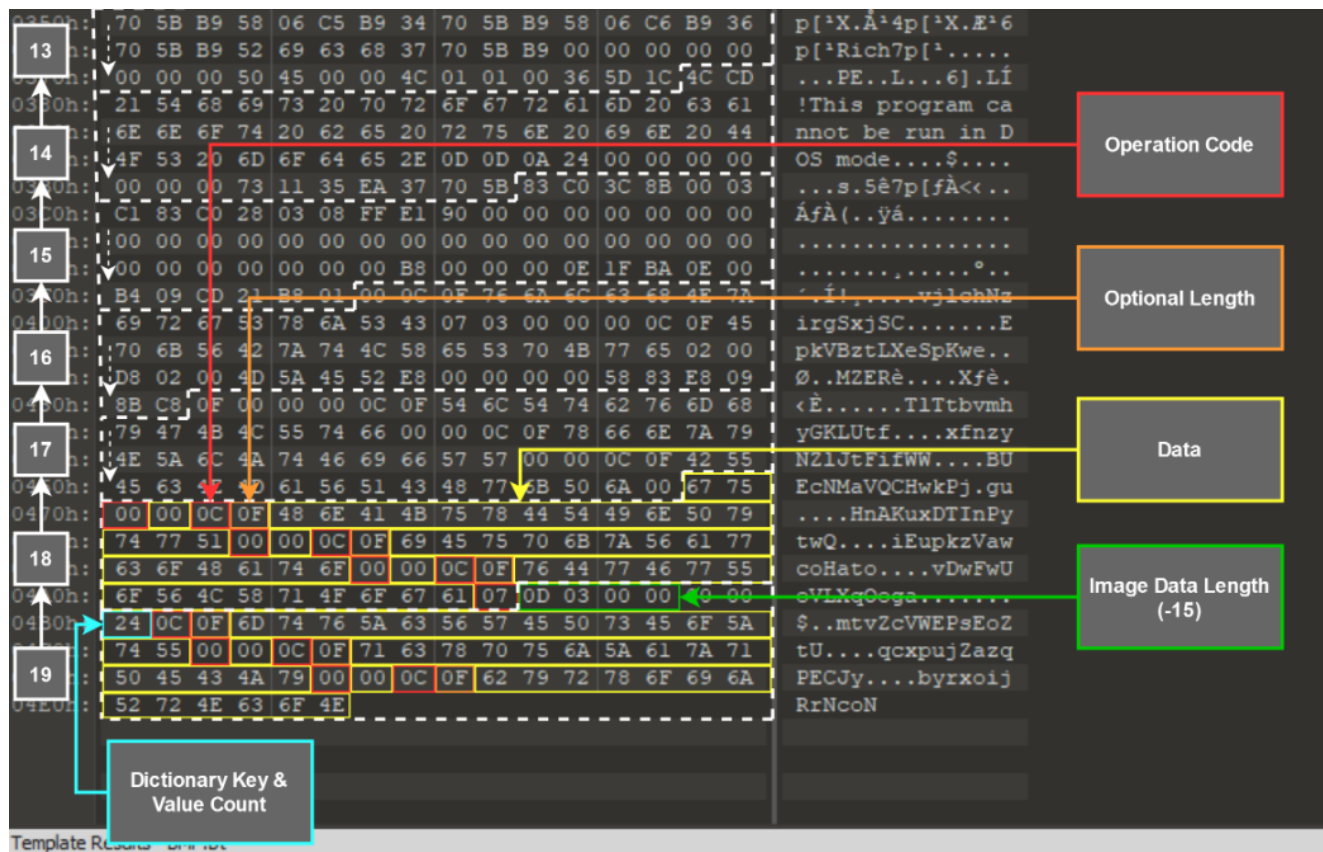
Figure 14: Partial dictionary encoded in a BMP image
