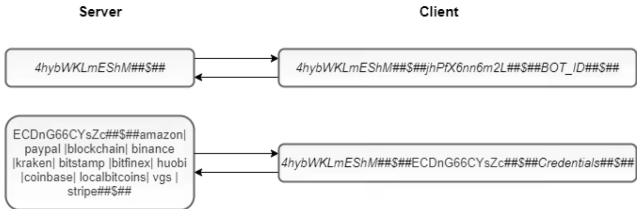
Figure 13: The decrypted communication between the client and the C&C server.
