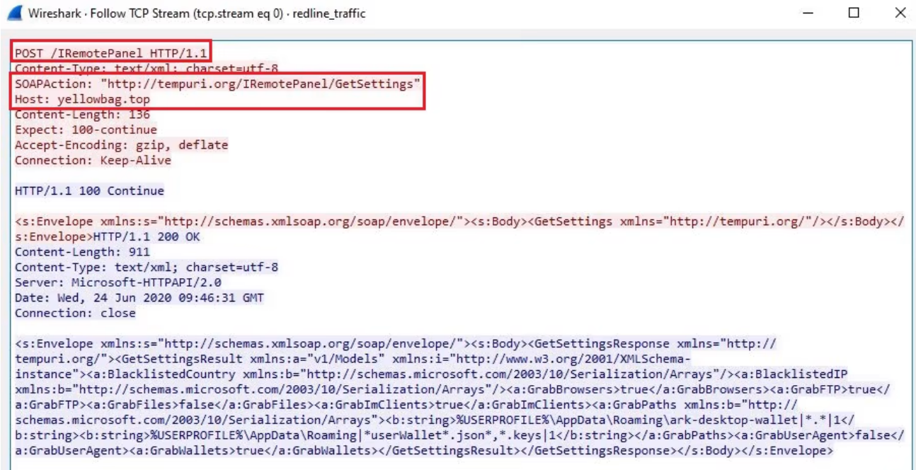
Figure 17: Fetching the client configuration settings.
