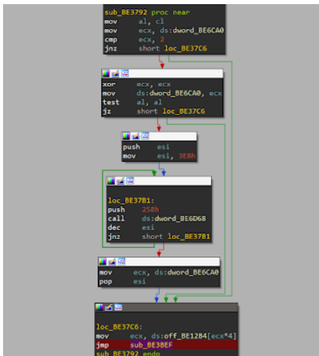
Figure 03 - Patched code used for decrypting C2 URLs.
