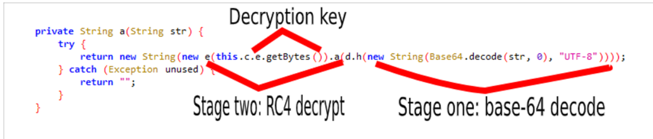
Figure 5: The decryption function, used throughout the program
