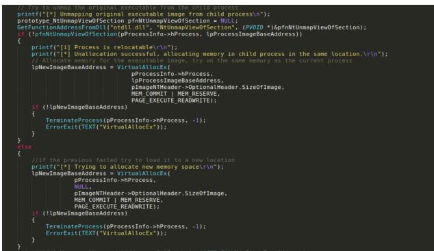
Unloading of the main module and then reallocating memory for the new executable in ProcessHollowing. Source code can be found <u>here</u>.
