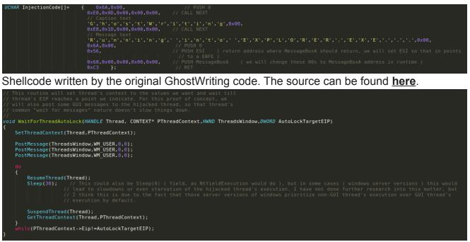
The main function that GhostWriting uses to continuously write desired content in target process. By setting registers in the thread context so they point to selected gadgets GhostWriting maintains control of the target process. PowerLoader and PowerLoaderEx
