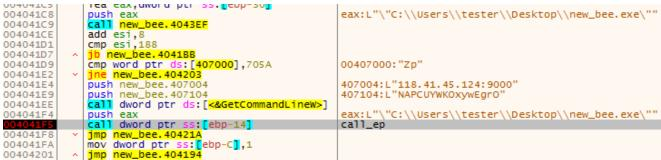
Calling the Entry Point of the manually-loaded NE module
