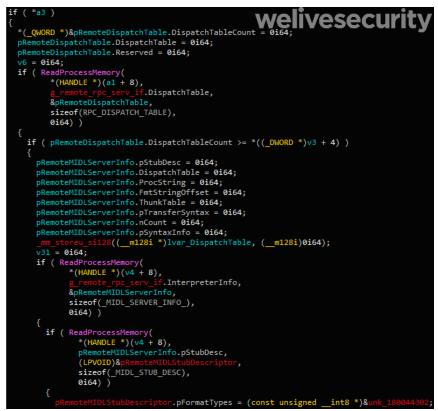
Figure 10. Snippet of code retrieving the RPC dispatch table of the current process (Hex-Rays screenshot)
