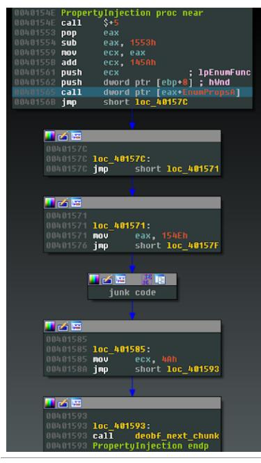
Fig. 3 - PROPagate Injection
