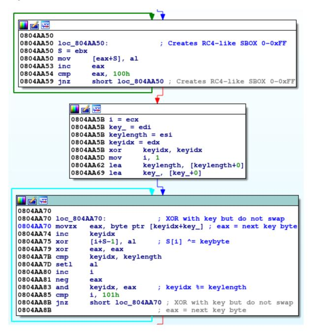
The RC4 initialization XORs the values in the permutation phase of the internal state initialization. As you can see in the last basic block, the code doesn't swap the values of S[i] and S[j] (compared to the RC4 pseudo code below).
