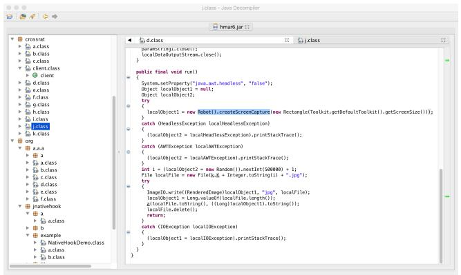
Via the java.awt.Robot().createScreenCapture the malware performs a screen capture, temporarily saves it as a disk (as a .jpg with a randomized name), before exfiltrating it to the C&C server.
