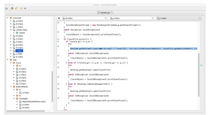
When the malware is executing on a Window machine, it will execute invoke rundll32 to load url.dll and invoke it's FileProtocolHandler method:
