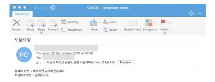
The email's attachments are two different HWP documents, both leveraging same vulnerability (CVE-2013-0808). This vulnerability targets the EPS (Encapsulated PostScript) format. The purpose of the shellcode is to download a payload from the Internet. The first email displays the following decoy document to the infected user and download the following payload:
