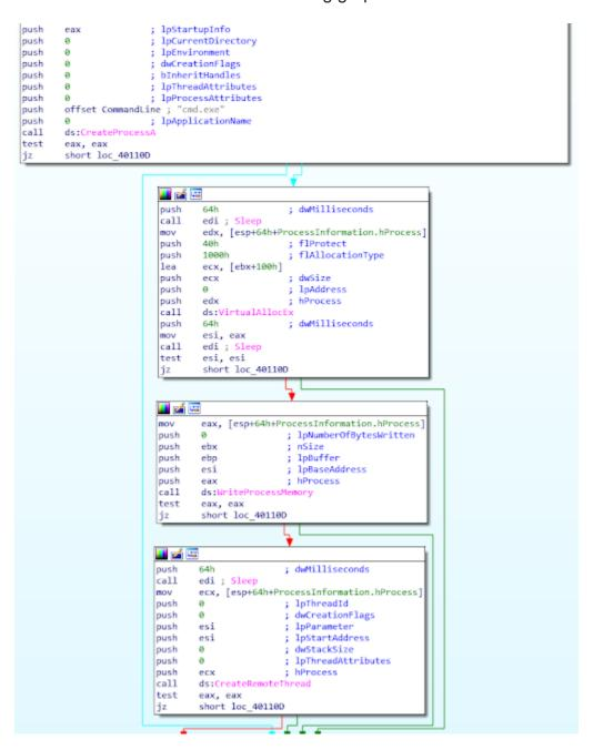
These execution steps allow the launch of the new ROKRAT variant by decoding the PE binary and injecting into the cmd.exe process.
