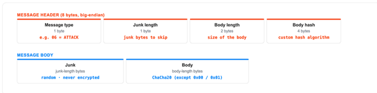
Figure 1 - Command anatomy for Aisuru C2 communication.
