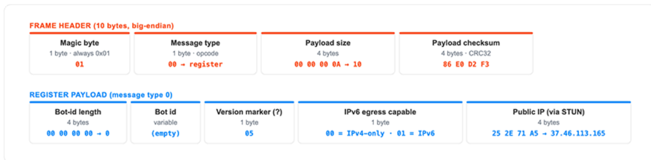
Figure 18 - Proxy bot's protocol framing.
