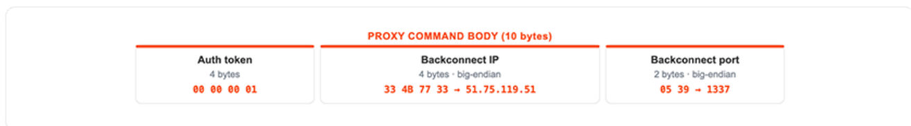
Figure 4 - Byte level view of the Aisuru proxy message.
