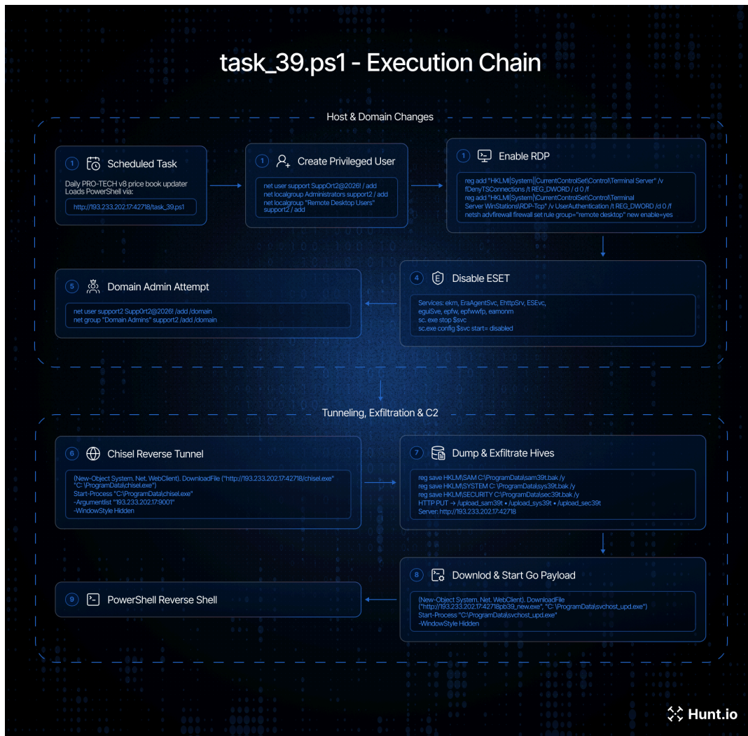
Figure 03: task_39.ps1 for account creation, defense impairment, credential theft, tunneling, payload staging, and an interactive shell To perform credential theft, the actor leveraged reg.exe to export registry hives to the C:\ProgramData directory. These were exfiltrated using the native PowerShell HTTP client, uploading to the C2 server with a PUT operation.
