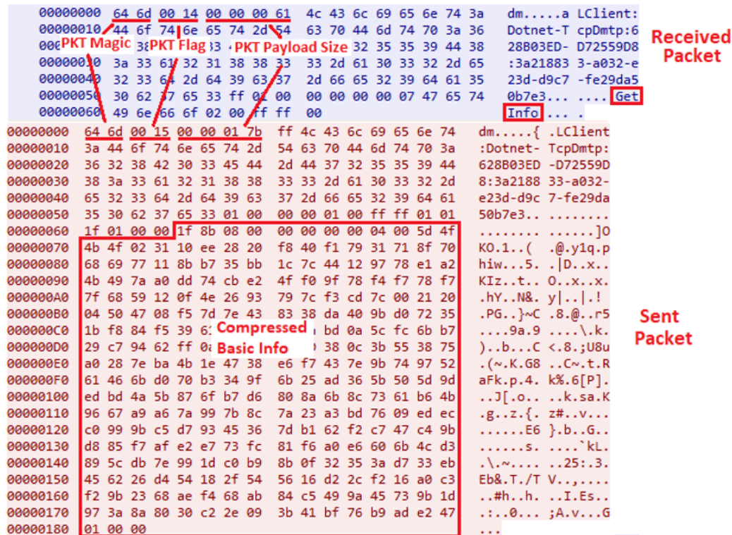
Figure 11: Calling the GetInfo() RPC. When the implant receives this 'GetInfo' RPC request, the Client.CommonService.GetInfo() method is called based on the RPC server's registry information. It sends the basic information stored in the Common.HostInfo variable, which contains the data as shown in Figure 12 below.
