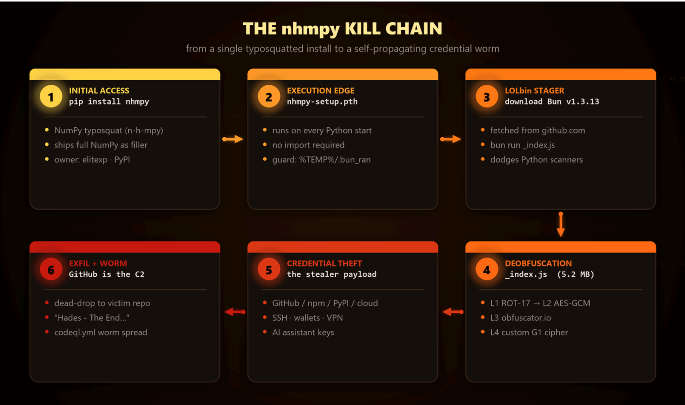
Figure 1: The full nhmpy kill chain — a single pip install typo escalates into a GitHub-borne credential worm.
