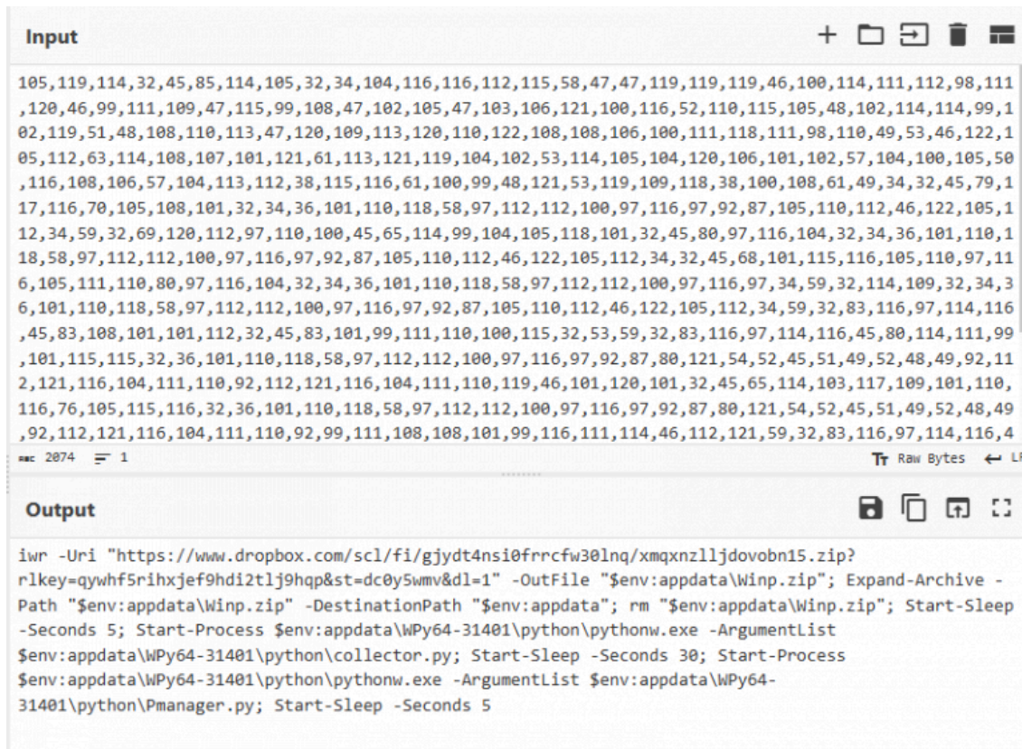
Fig4: Decoded Powershell command from CyberChef
