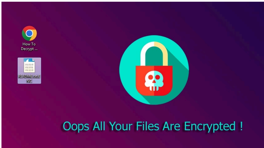
Figure 19: Desktop Image changed. Filename: "How To Decrypt My Files.html" dropped to Desktop. Encrypted files have .ENC extension.
