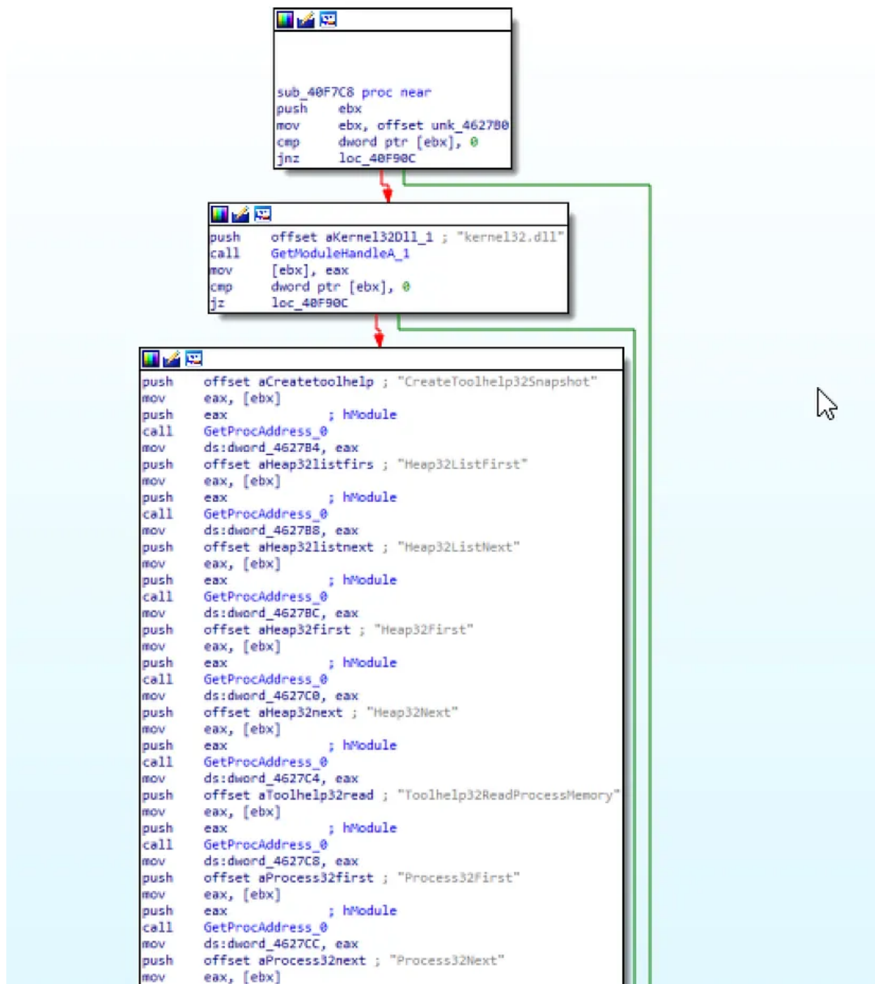
ToolHelp32 APIs resolved at runtime to enumerate system components
