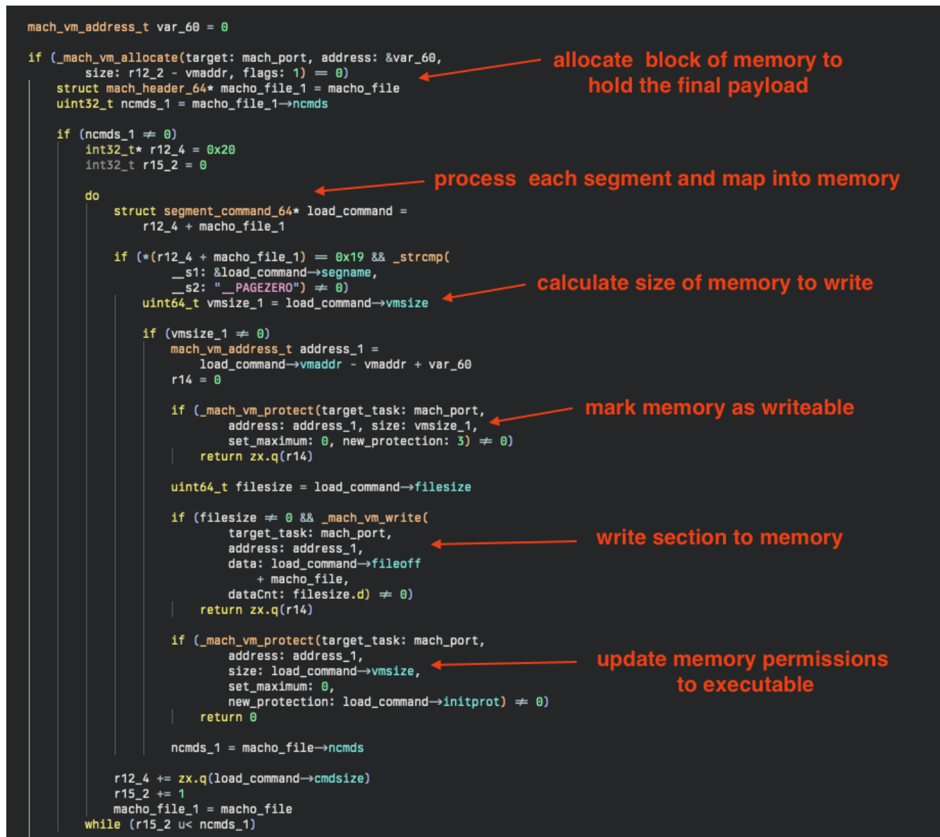
Figure 28: Decompilation of the memory protection modifications per segment
