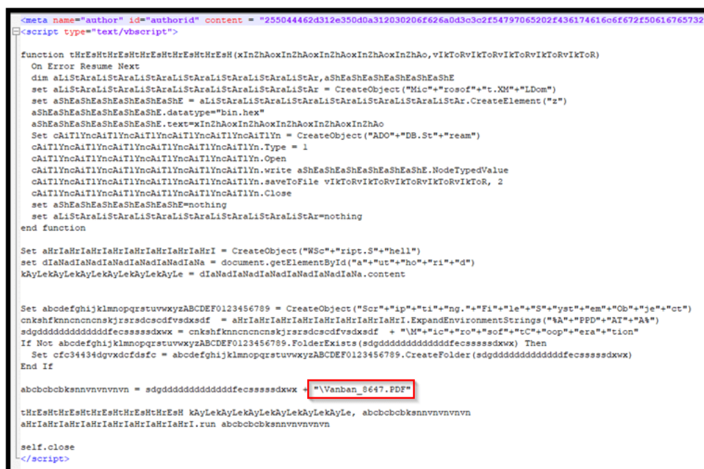
After completing DLL sideloading, the "Vanban_8647.PDF.ps1" script executes the "Vanban_8647.PDF.hta" file, which extracts a lengthy hexadecimal string from a meta tag within the HTA file. This hexadecimal string is then decoded into its binary form, which is saved as a PDF file named "Vanban_8647.PDF" in the directory "C:\Users\<user>\AppData\Roaming\Microsoft\Cooperation\". Subsequently, the PDF file is opened. The figure below shows the contents of the "Vanban_8647.PDF.hta" file.
