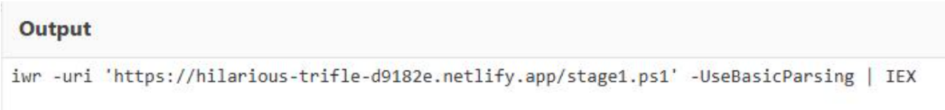
Figure 4. The deobfuscated code that executes the same PowerShell command as Figure 3.
