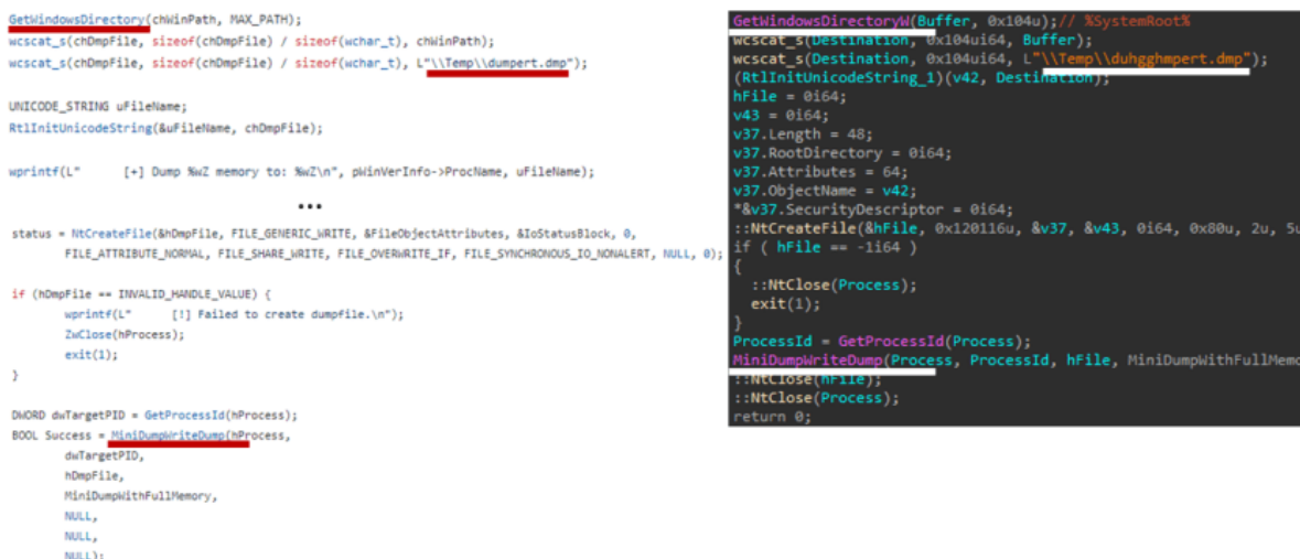
[Figure 7] Left (Dumpert open source) vs Right (Dumper used by Dalbit group)
