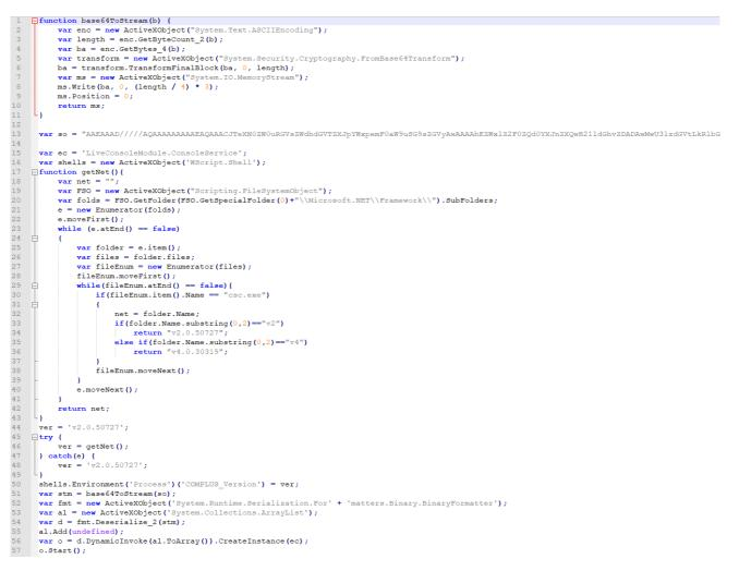
The JS code also reflectively loads LiveConsoleModule.dll in the memory. This dll is actually a remote Shell RAT, which listens to the local TCP port 12323 and uses cmd to execute remote Shell commands.
