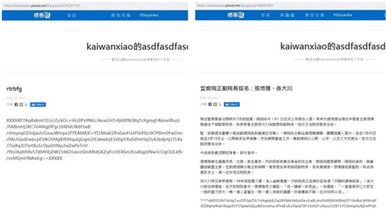
Figure 10. Taleret configuration (left) and Comeon downloader payload (Roudan, right) on the same blog
