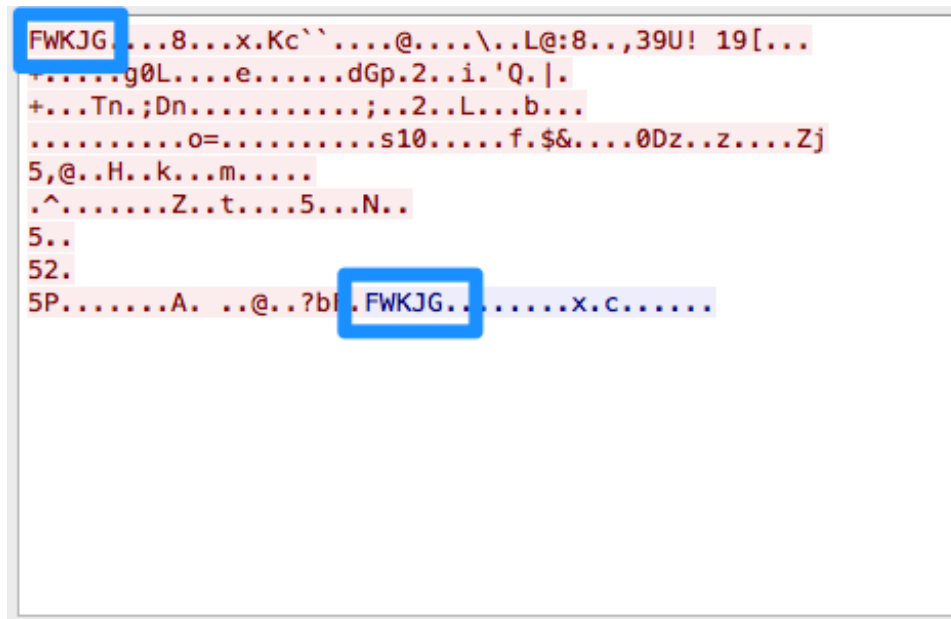
Figure 1. Gh0st “magic tag” value sent over custom TCP protocol
