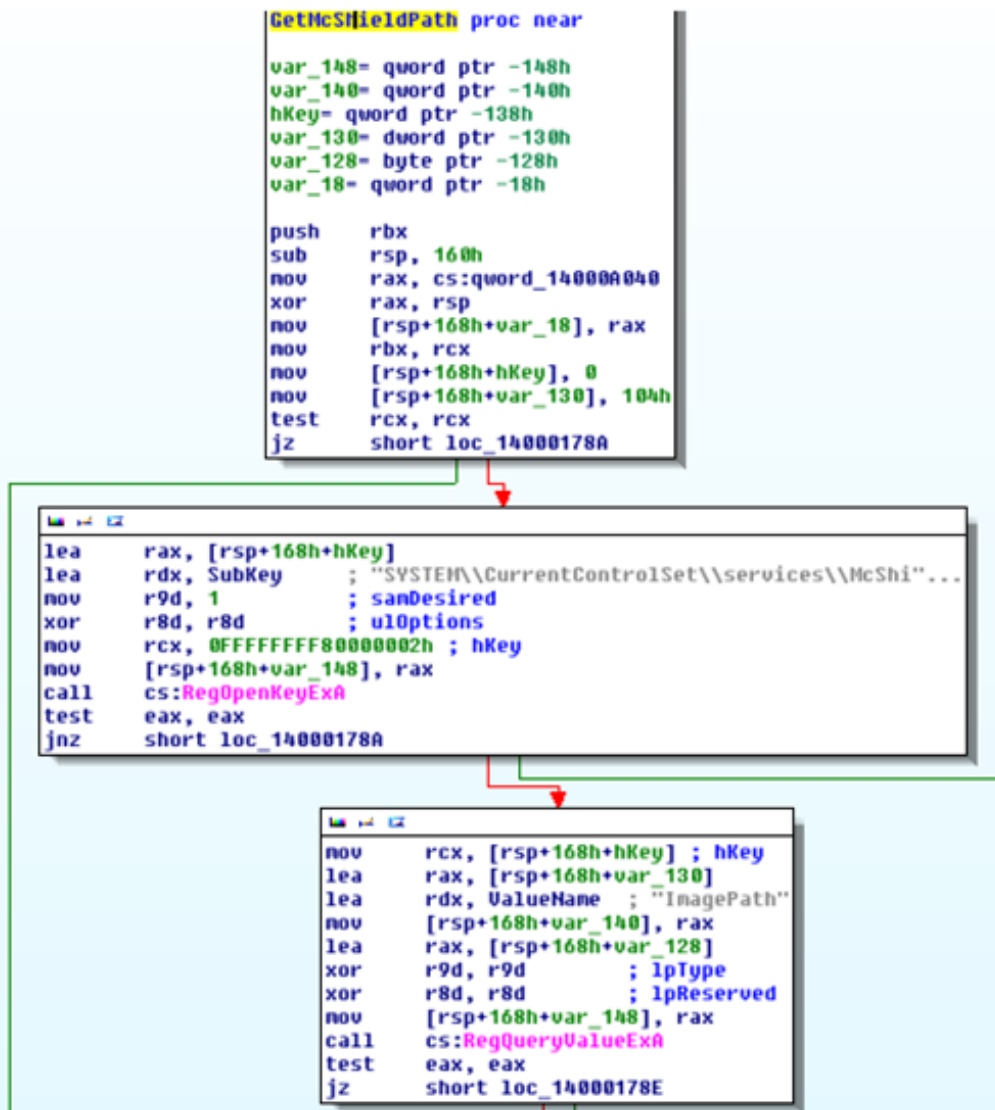
Figure 2. BKDR64_WIPALL.F obtains the Image Path of McShield.exe from the registry's list of services: HKLM\CurrentControlSet\services\McShield
